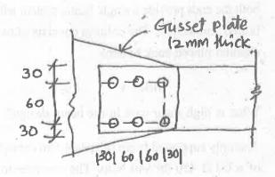
(c) A single angle member carries a factored axial load of 400 kN. Design the member and the connection with the gusset plate 10 mm thick use Fe 410 grade steel.
